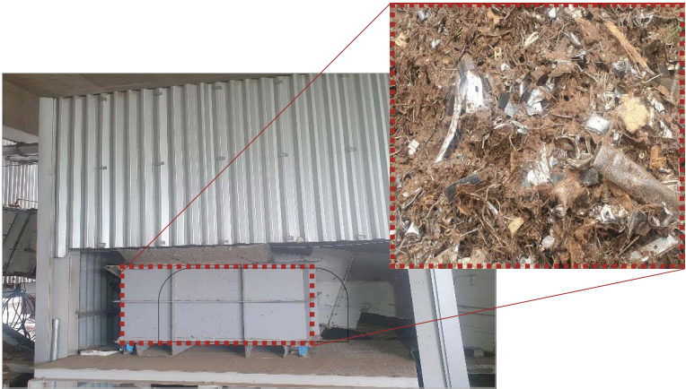
Magnetic Separator: A device that selects only substances that adhere to a magnet from within a mixture
