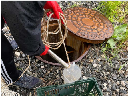
Water quality analysis sampling at non-point pollution reduction facility
