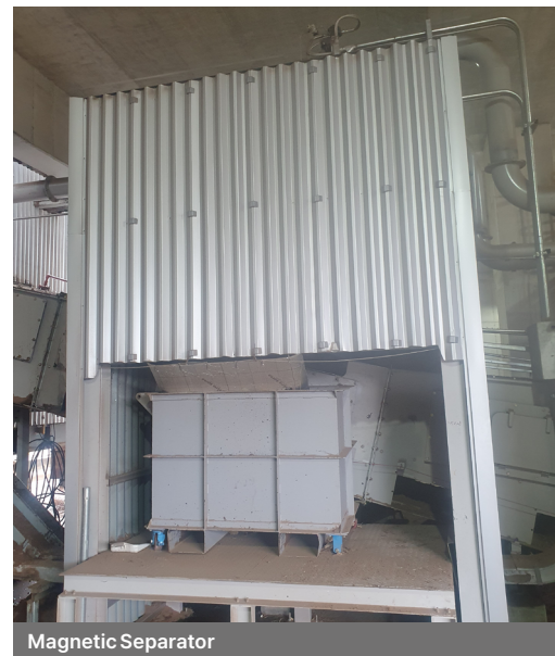
*Magnetic Separator: A device that separates magnetic materials from a mixture.
